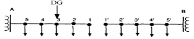
Fig. 2 Tie switch location in a two feeder example
