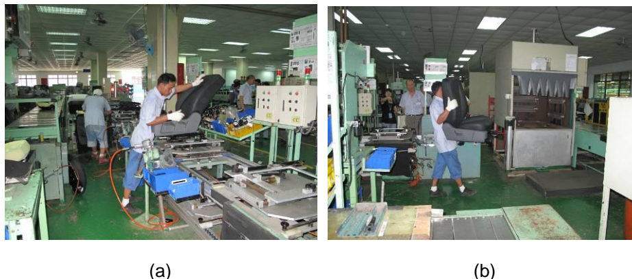
Fig 3. (a) The final assembly of covering the form material with external vinyl upholstery. (b) The worker carries the final assembly of the driver's seat to the oven for temperature set-ting.
